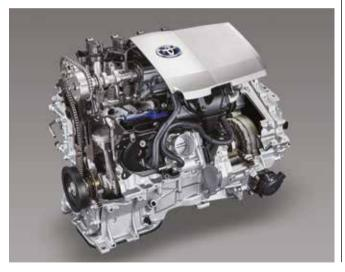
High tumble flow has been achieved through the shape of the intake port and the piston, enhancing EGR (Exhaust Gas Recirculation) and improving combustion. A diagonal squish combustion chamber aligned with the spark plug angle improved anti-knock performance and fuel efficiency. The EGR (Exhaust Gas Recirculation) system valve has been enlarged to optimise gas flow, the intake manifold gas distribution structure has been optimised and EGR cooler heat exchange efficiency has been increased.
