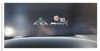
**Head-Up Display (HUD):** Its position and brightness adjustable via the steering wheel switchgear, an optional 10" colour TFT Head-Up Display –the largest in the segment– projects various driving-related information and warnings onto the windscreen glass within the driver's field of view, such as speed limits, navigation prompts and an eco-driving indicator.
