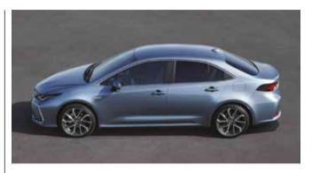
Its overall length increased by 10 mm, the new Sedan features a 5 mm reduction in front overhang and a 15 mm increase in rear overhang. It shares the same extended 2,700 mm wheelbase as the Touring Sports.
