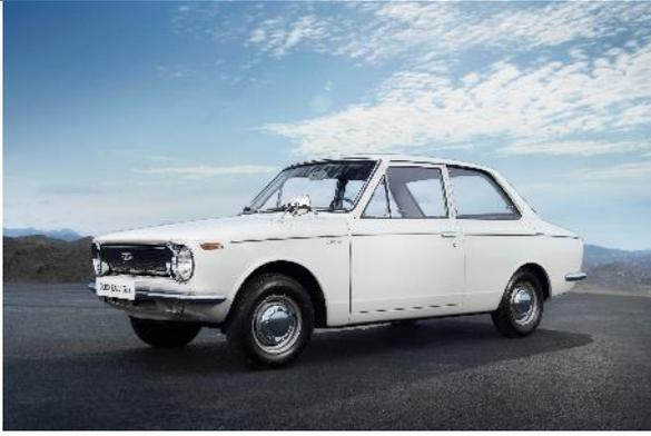
variety of body styles and adopted many new technologies not seen on the Japanese market before, such as MacPherson strut suspension and a four speed transmission. The model line-up consisted of a two-door saloon, four-door saloon and a two-door estate.
