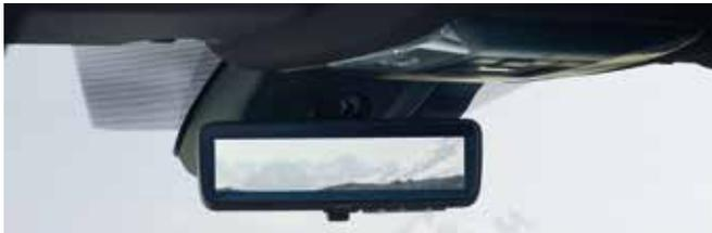
in the load space or tall rear-seat passengers obscure the driver's line of sight. The camera also provides a wider field of vision and the driver can use touch controls to adjust the image, including a zoom function.
