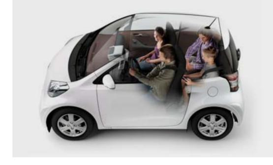
All desired cabin comforts are housed within the iQ's 2,000 mm wheelbase. A distance of 710 mm is maintained between the driver and front passenger seat, giving space that is comparable to that of a C-segment vehicle.
