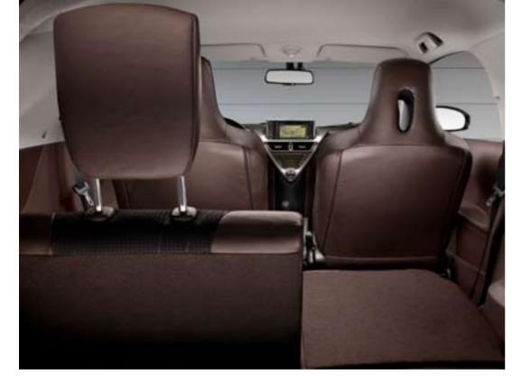
The front pillars are positioned forward and then slope back to eliminate any feeling of claustrophobia. The front passenger seat can be slid forward to ensure enough legroom to accommodate three 190 cm tall adults and one child or luggage. Both rear seats can be folded down to increase the load capacity of the boot to a max of 238 litres (VDA) or 32 litres when both the rear seats are in position.
