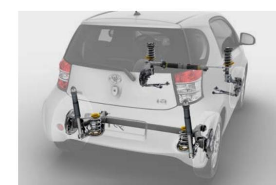
The MacPherson strut front suspension features a high 8.3° caster angle for more toe-out when lateral forces are applied, which basically means a more stable stance for the front wheels. By decreasing the stiffness of the steering arm, toe-out is added too when lateral forces increase, thus again adding to a high degree of stability. Both measures increase understeer and add to stability. Optimised geometry and damping force achieve maximum ride comfort and driving stability.
